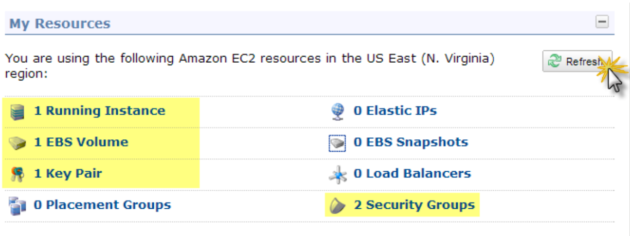
Figure 18: After launching an instance, the My Resources pane shows there is one running instance along with one EBS (Elastic Block Storage) volume, one key pair, and two security groups.
