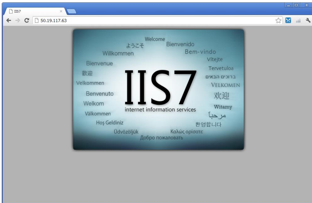
Figure 40: After you associate an elastic IP address with your server instance, your server is accessible from the outside world – subject to the rules in its security group.
