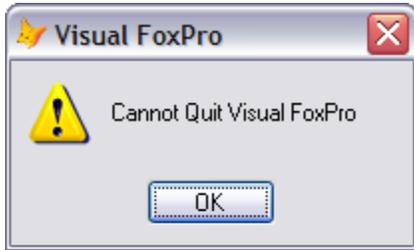
**Figure 3: The "Cannot Quit Visual FoxPro" condition occurs if you try to shut down VFP while an event loop is still active.**
