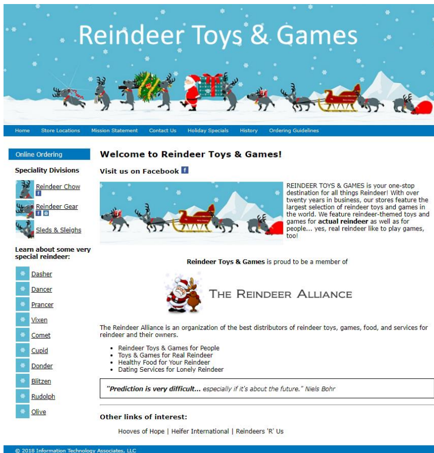
Figure 4: The original website was designed for desktop browsers with a viewport at least 950px wide.
