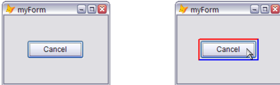
Figure 8: A sample form with the MouseOver Effects foundation class applied to the Cancel button. The effect is off, as shown on the left, and appears only when the mouse moves over the control, as shown on the right.
