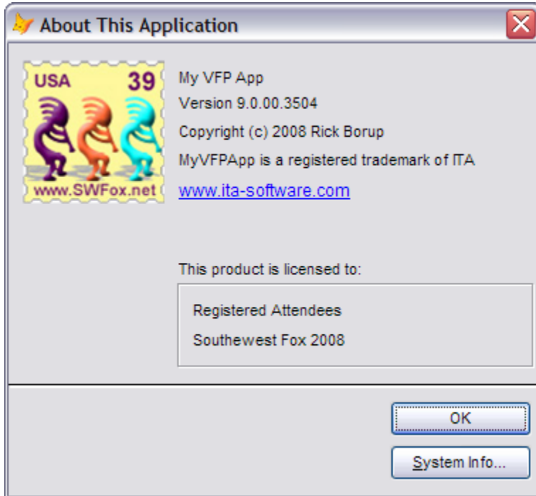
Figure 12: This About form uses the File Version foundation class to retrieve the version number from the program being executed.
