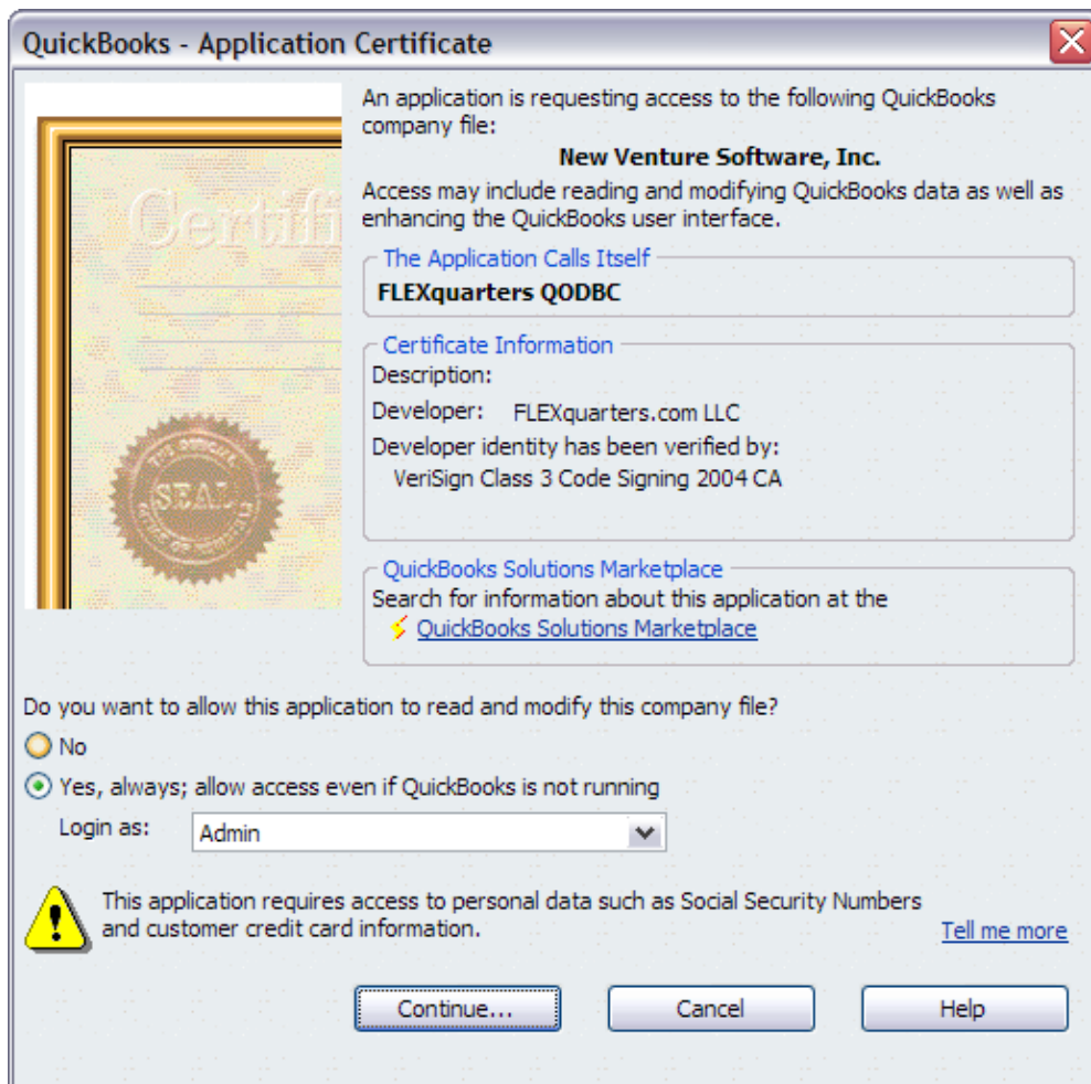
Figure 4: The first time you connect to a company file using QODBC, you need to tell QuickBooks to allow access.
